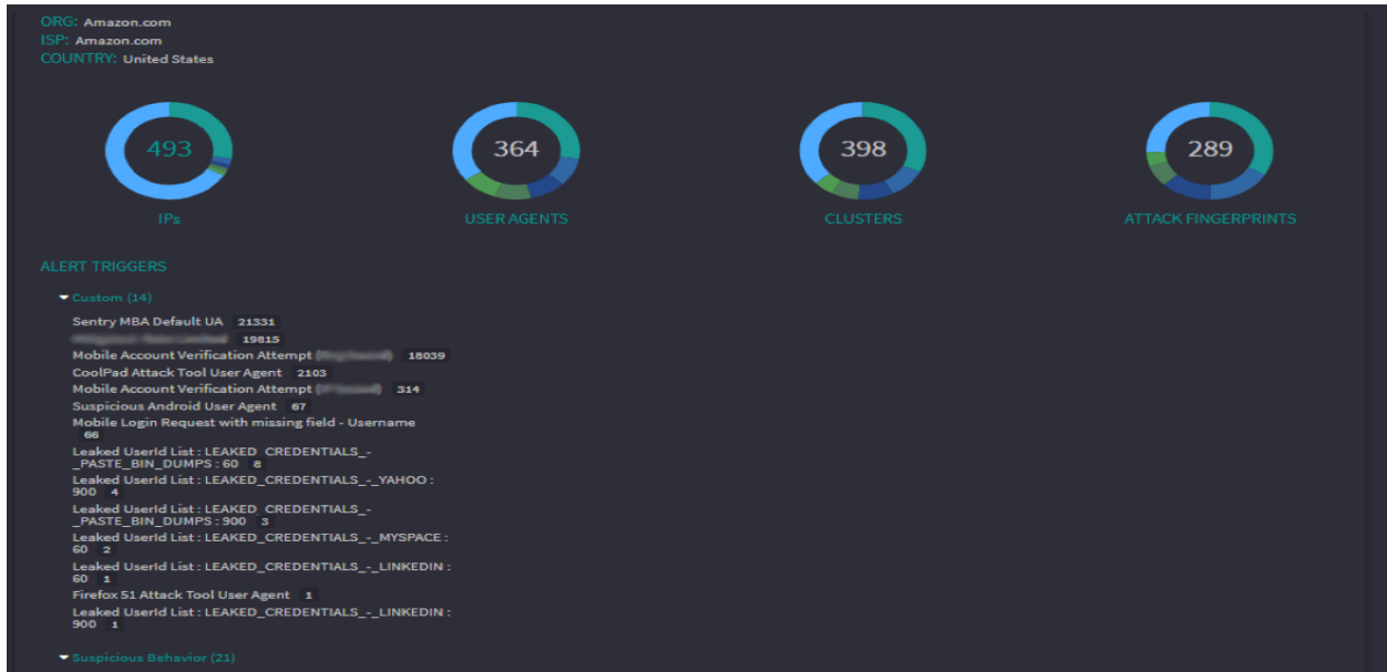
Figure 1: Details of an attack cluster using AWS as a proxy to launch the attack. Attackers will try to blend in with legitimate traffic from high reputation cloud providers, but signatures of attack tools and the presence of stolen credentials are suspicious. This attacker rotated through over 364 User Agent strings from 493 IP addresses.
